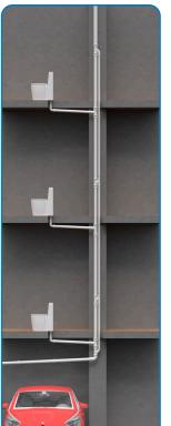
**Molecor** has designed this new ventilation part in accordance with the CTE (Spanish Technical Building Code) regulations on ventilation systems in buildings with more than 7 floors, although its use is recommended in any type of installation.
